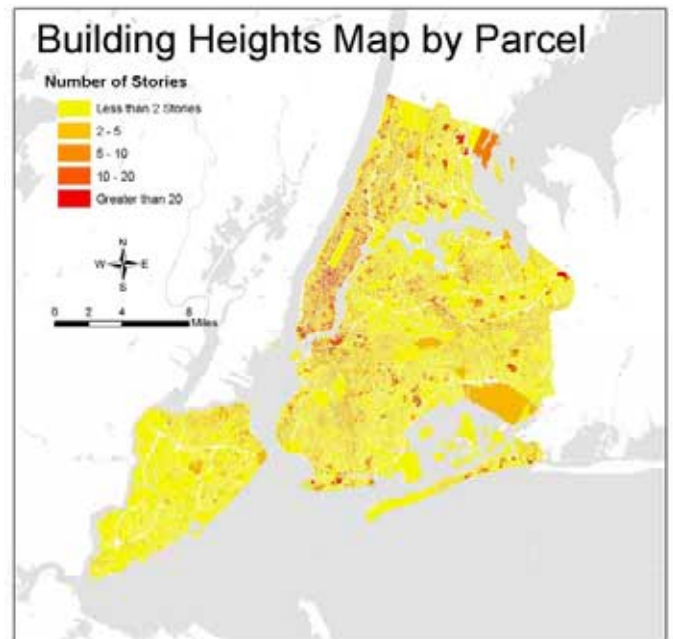
Figure 2-7. Average building height derived from number of stories. Extracted from the real property database of New York City’s Department of Finance, 2002.
